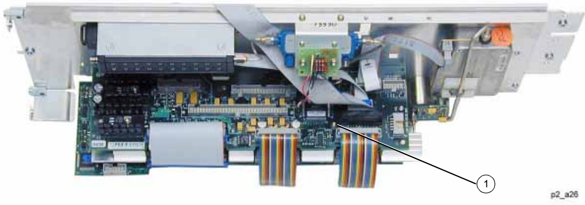
Figure 3-21 E8267C Microcircuit Interface Deck Top View
