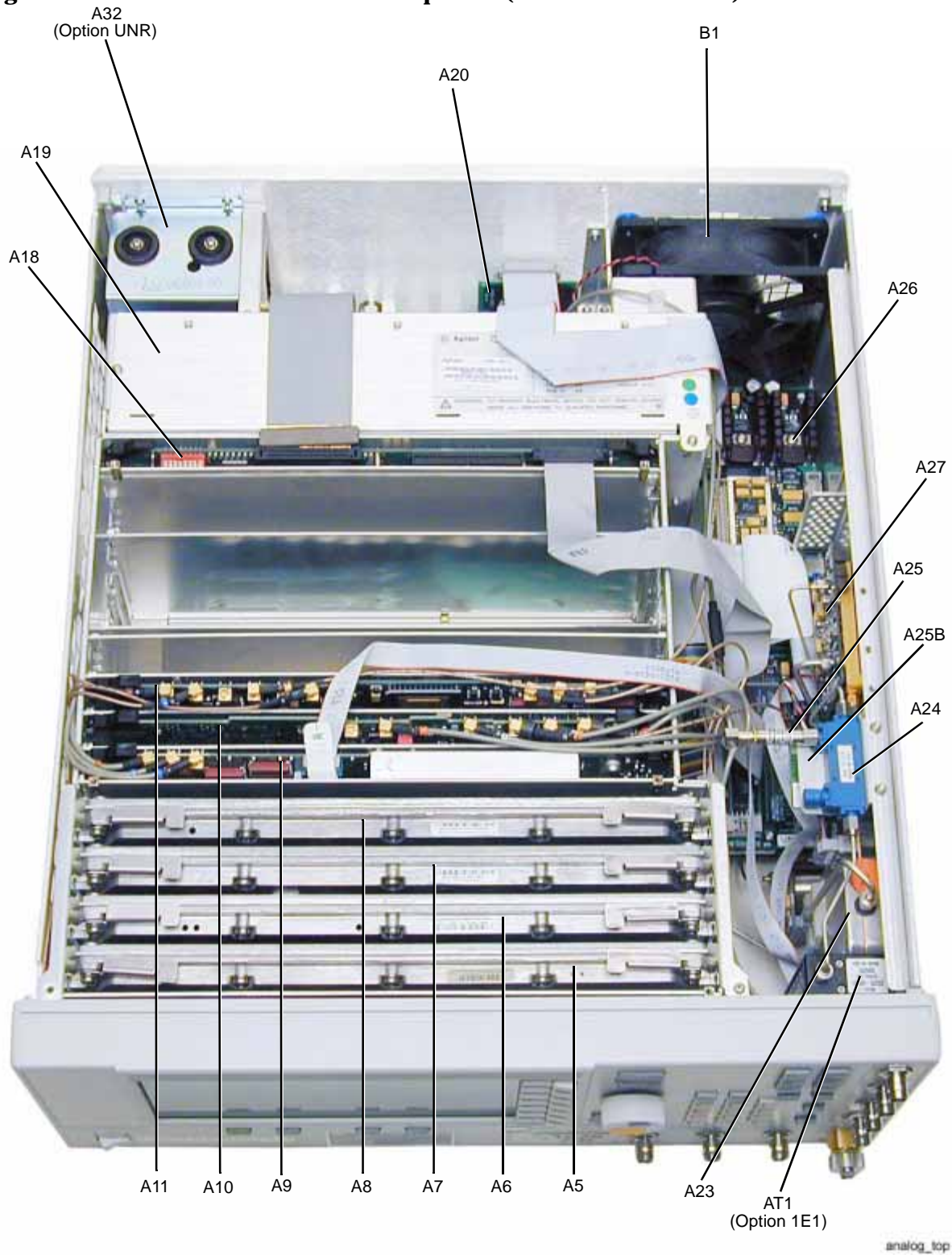
Figure 3-3 Assemblies from a Top View (E8247C and E8257C)
