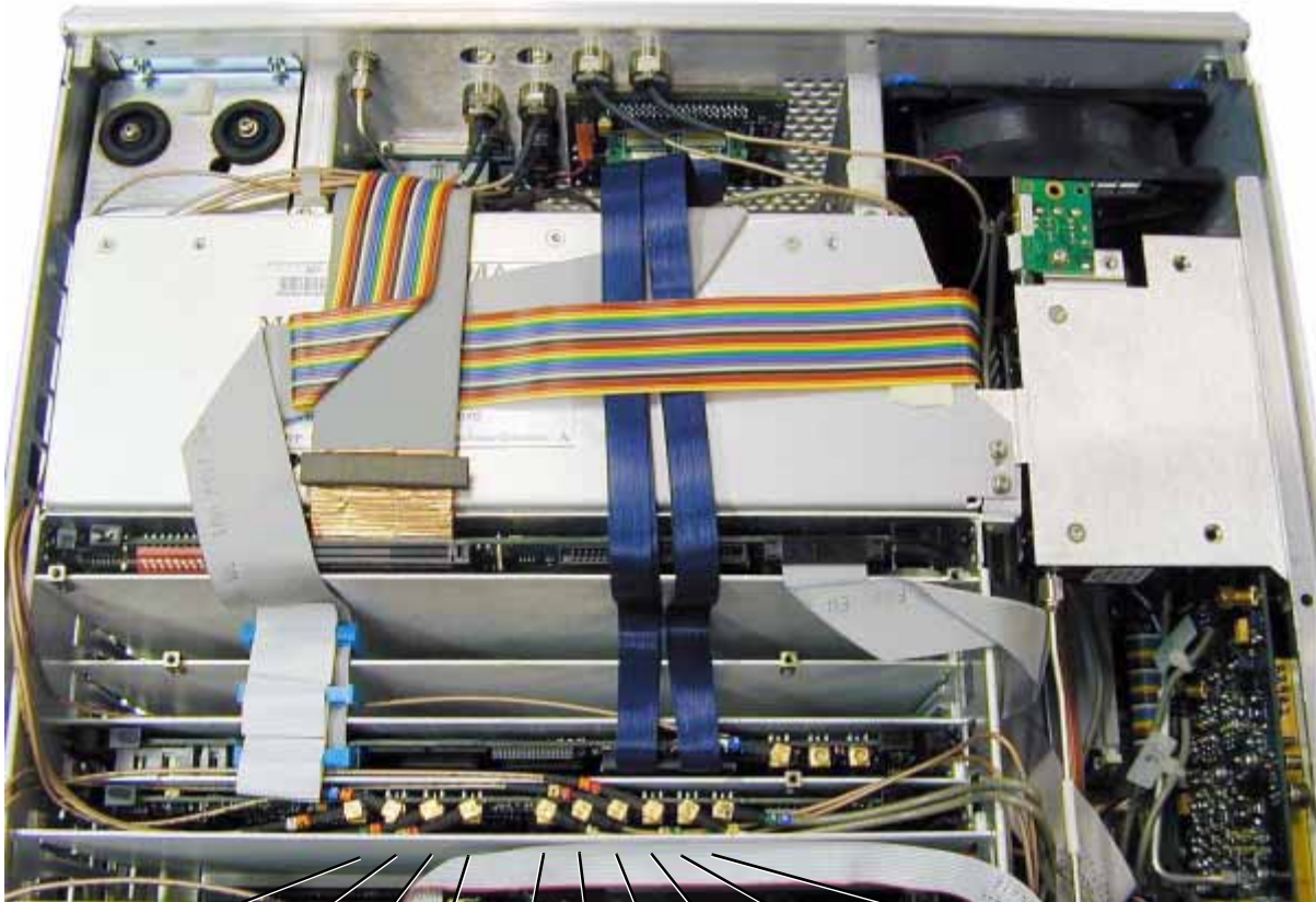
Figure 2-46 A35 3-20 GHz I/Q Modulator
