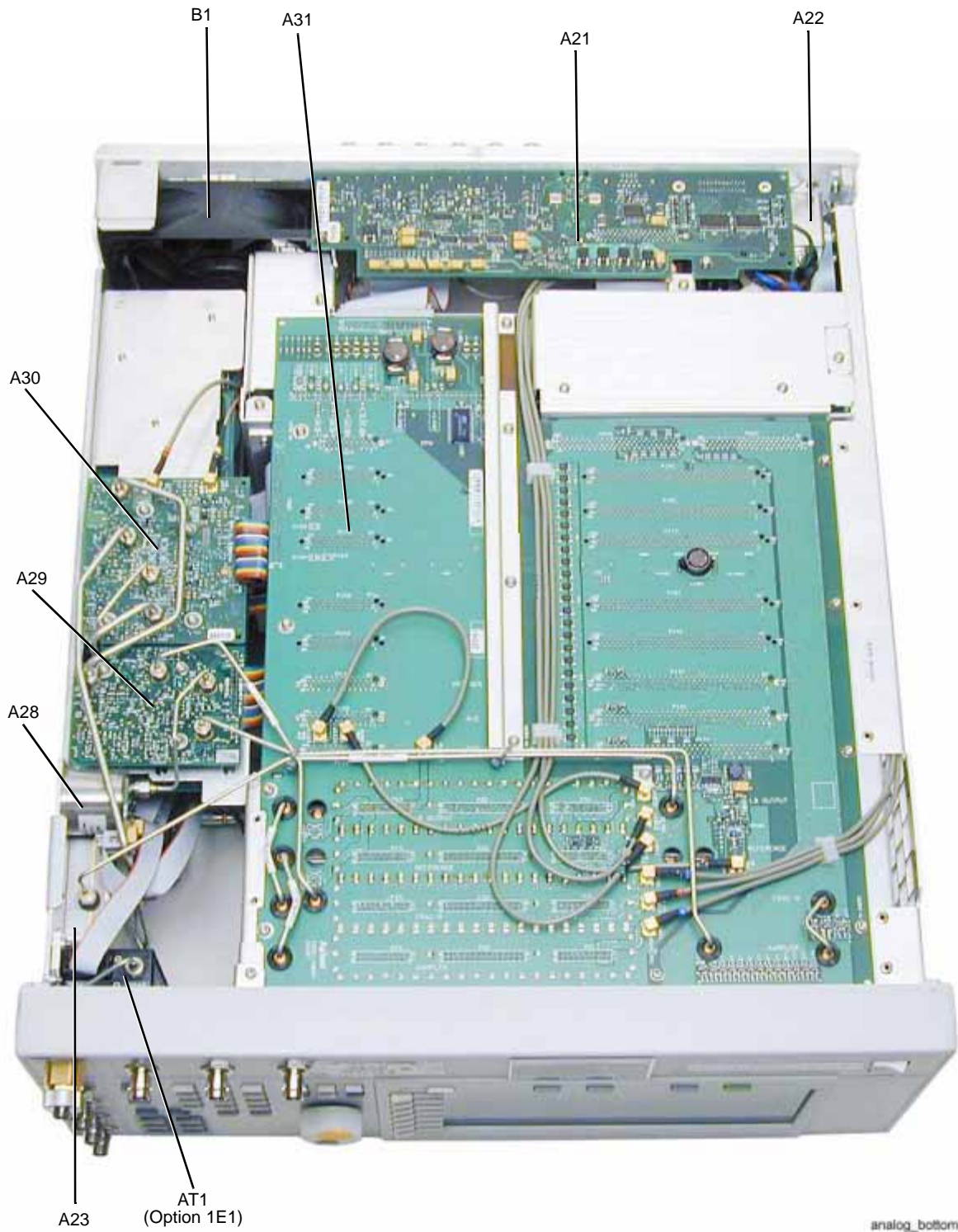
Figure 3-9 Assemblies from a Bottom View (E8247C and E8257C)
